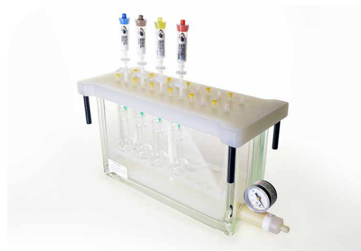
SiliaFast FaPEX can be used with a SPE vacuum manifold
