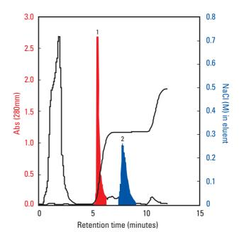
Column: TSKgel BioAssist S, 7  $\mu$ m, 4.6 mm ID x 5 cm L; Mobile phase: 20 mmol/L sodium phosphate buffer, pH 6.0; Gradient: 0 mol/L - 0.3 mol/L NaCl (5 min), 0.3 mol/L - 0.5 mol/L NaCl (10 min); Flow rate: 1 mL/min; Detection: UV @ 280 nm; Sample: 500  $\mu$ L of 9.5 mg/mL lgM in mouse ascites fluid; shaded peaks represent albumin and lgM respectively
