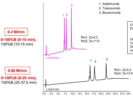
Column : BioPro HIC BF 4 µm, 100 X 4.6 mml.D. Eluent : A) 100 mM NaH<sub>2</sub>PO<sub>4</sub>-Na<sub>2</sub>HPO<sub>4</sub> (pH 7.0)
