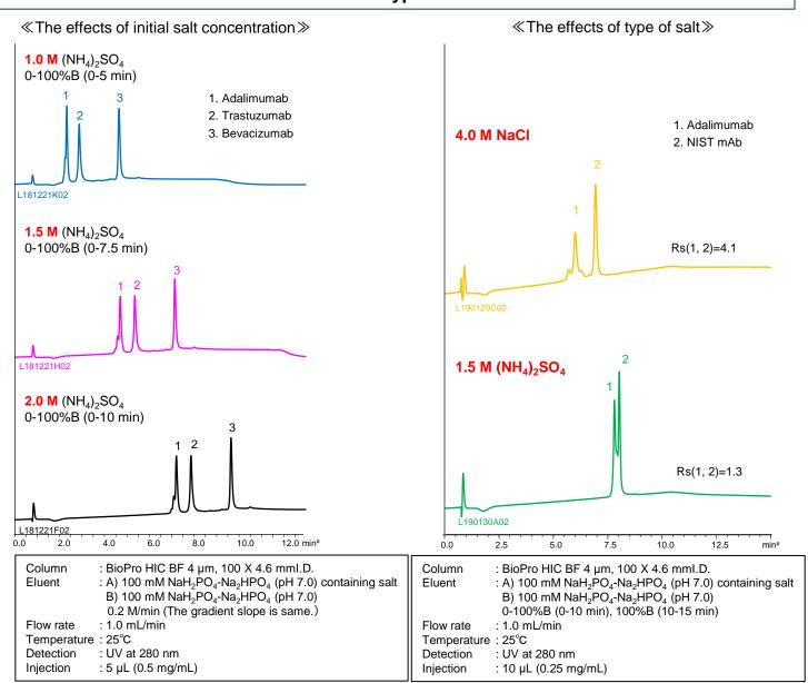
The buffer containing  $(NH_4)_2SO_4$  is often used as mobile phase of HIC because  $(NH_4)_2SO_4$  has strong salting-out effect. The higher the concentration of initial  $(NH_4)_2SO_4$ , the stronger retention of proteins, so a buffer with high salt concentration is effective for separation of the low hydrophobic proteins with weak retention.
