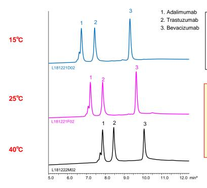
$\begin{array}{ll} \mbox{Column} &: \mbox{BioPro HIC BF 4} \ \mbox{$\mu m, 100 X 4.6 mml.D.} \\ \mbox{Eluent} &: \mbox{$A$)} \ 100 \ \mbox{mM NaH}_2\mbox{PO}_4\mbox{-Na}_2\mbox{HPO}_4 \ \mbox{(pH 7.0)} \\ \end{array}$
