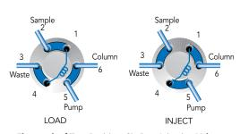
Flow path of Two-Position, Six-Port Injection Valve
