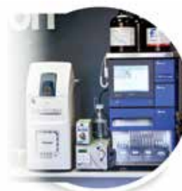
Online Flash/CMS – mass directed fraction collection
